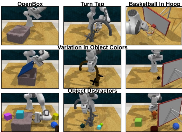
Fig. 8. We modify the original RL Bench environments to introduce color variations and add distractors.
