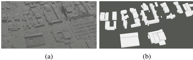
Fig. 4: Study area: (a) aerial LiDAR point cloud, (b) 3D building models reconstructed with City3D [22]
