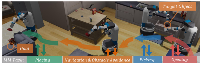
Fig. 1. An illustration of a goal-oriented MM task, which is multi-stage and requires learning heterogeneous behaviors such as navigation, collision avoidance, picking, placing, and opening concurrently.
