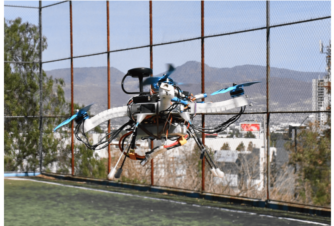
Fig. 1: QuadSoft prototype during outdoor flight. The four arms are tendon-driven and flexible, actuated by servomotors to enable in-flight morphological adaptation.
