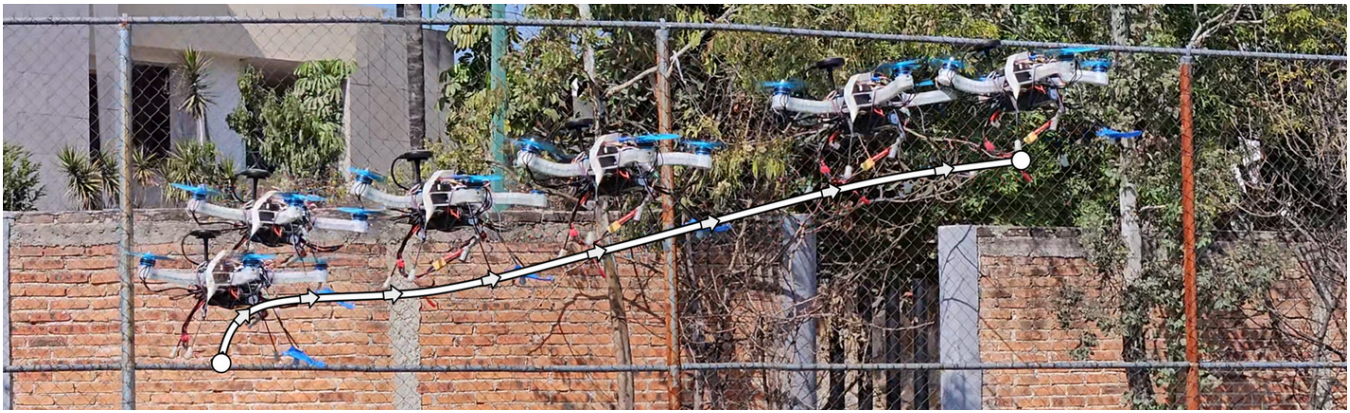
Fig. 7: Sequence of an outdoor flight demonstrating forward displacement generated by tendon-driven arm actuation under altitude hold. The snapshots illustrate the QuadSoft’s trajectory during morphological reconfiguration, highlighting controlled horizontal motion achieved without affecting altitude.
