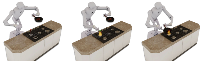
Fig. 4. The steps of a steak cooking task. The robot must approach the stove (left), toggle on the stove by pressing the button (center), place the pan on the heat source affordance (right), and wait for the steak to cook.
