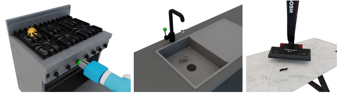
Fig. 1. Simulation Affordances are needed for simulating a variety of features that are necessary for household robotics. Left: toggle button and heat source affordances are used to simulate a stove. Center: toggle button and fluid source affordances are used to simulate a faucet. Right: toggle button and particle remover affordances are used to simulate a vacuum cleaner.
