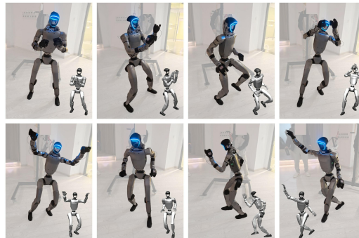
Fig. 9. Snapshots of the learned dancing motion using A2CF on the real robot. Each subfigure includes the corresponding target motion from the LAFAN1 dataset (bottom right) for side-by-side comparison, highlighting the high-fidelity reproduction of complex body dynamics.
