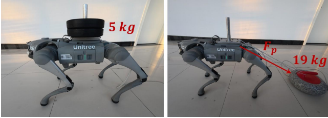
Fig. 6. Diagram of the real world ablation experiment setup. Left: The robot carries a 5 kg payload. Right: The robot pulls a 19 kg weight via a rope to simulate pulling disturbance.
