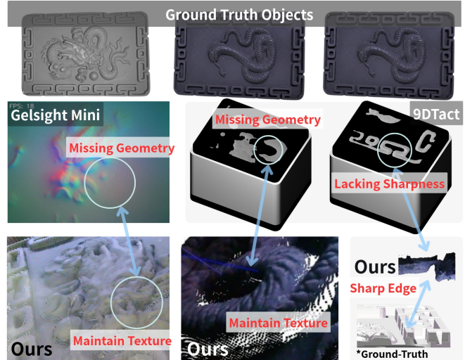
(b) Limitations of coated VBTS in perceiving recessed geometry.
