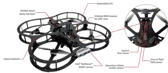
Fig. 3. QDrone2 hardware platform with equipped sensors.
