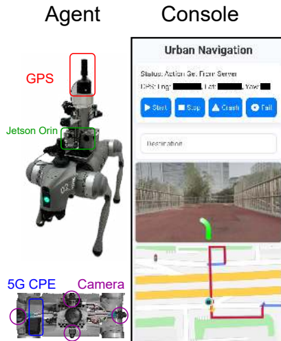
Fig. 3: Real-world deployment of UrbanVLA. Our system consists of a quadruped robot equipped with GPS, Wi-Fi, a camera, and an onboard computing unit, along with a mobile-deployable console for real-time monitoring, sending navigation targets, visualizing maps and model predictions, and annotating teleoperation data used for reinforcement learning.
