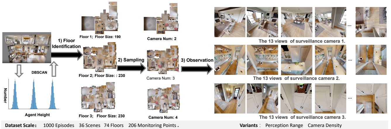
Fig. 2: The surveillance camera observation generation pipeline, consisting of (a) floor identification, (b) camera sampling, and (c) observation configuration.
