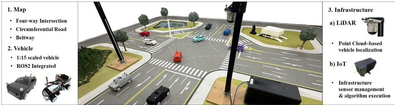
Fig. 1: Main components of CIVAT
