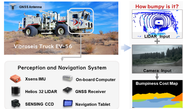
Fig. 1. A typical scenario in field operation environments. Equipped with an onboard perception system, the EV-56 truck can successfully predict the cost of terrain bumps in its surroundings using our proposed online learning framework.
