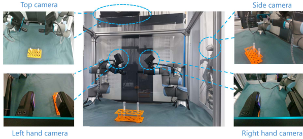
Fig. 3. Dual UR3 experimental setup with four cameras (Top: Kinect; Side: D435i; Wrists: D405) and custom grippers.
