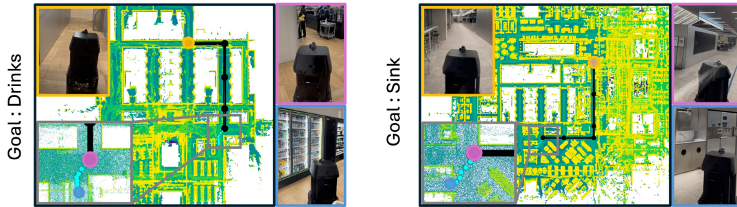
Fig. 5. Visualization of real-world experiments. ●: Start pose, representing the initial position from which navigation is initiated. ●: Coarse goal pose, selected based on its language embedding similarity to the target object. ●: Optimized goal pose, which is obtained through optimization of the implicit language map, ensuring that the target object is accurately brought into view.
