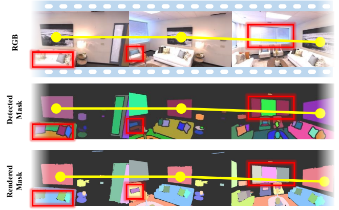
Fig. 4: The comparison between rendered and detected masks highlights its effectiveness in associating instances across frames (yellow lines) and mitigating missing, under-, or over-segmentation (red boxes).
