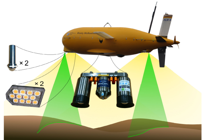
FIGURE 6. BioCam setup on ALR. The main housing containing the cameras and electronics is mounted centrally. Sheet lasers and LED strobes are mounted one each at the front and the back of the vehicle.
