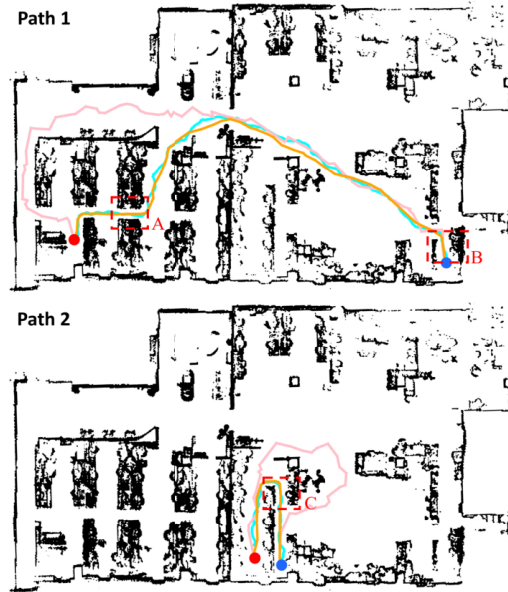
Fig. 19. Global path planning results in a 40m×25m laboratory using the RoA-Planner (orange), Art-Planner (pink), and TRG-Planner (cyan). The environment includes a mix of narrow corridors and open fields. The width of region A is approximately 0.8m, and that of region C is approximately 1m.
