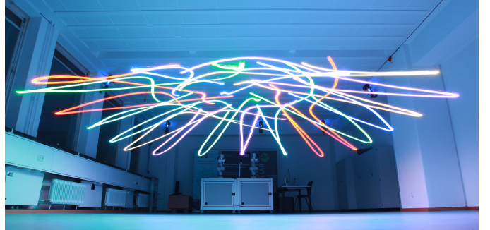
(a) Long-exposure image of 12 drones transitioning from a helix to a spiral motion at a musical beat.
