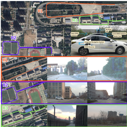
Fig. 3. Data collection vehicle sensor configuration and satellite images of recorded driving routes. There are three routes being recorded in total at Chang'an University, Xi'an, China. Route 1 (R1) is shown in red trajectory, Route 2 (R2) is shown in purple trajectory, while Route 3 (R3) is shown in green trajectory.
