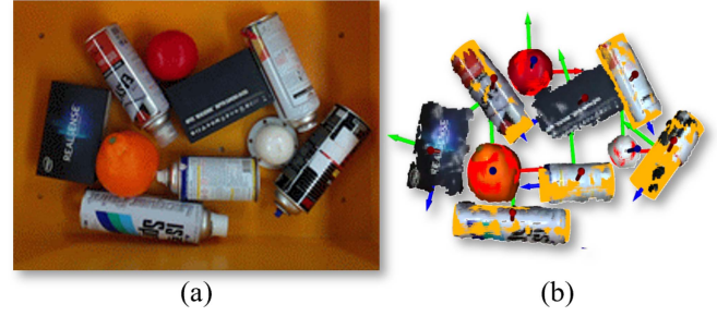
Fig. 3. Primitive shape fitting result in cluttered bin environments. (a) RGB image of cluttered scenes with various unknown objects. (b) Estimated primitive shapes with their poses overlaid. (Cylinder: Yellow, Sphere: Red) Despite heavy occlusion and object diversity, our shape matching module robustly decomposes and estimates the pose of each item without requiring mesh models.
