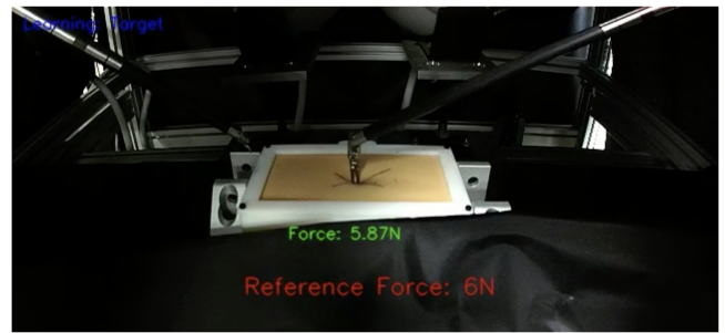
Fig. 5. Study participant's stereoscopic camera view of the patient side of the dVRK through the visual console. The phantom tissue-sensor enclosure is placed in the center of the workspace. During the experiment, participants palpate the center of the tissue pad with the tip of the ProGrasp forceps attached to the PSM.
