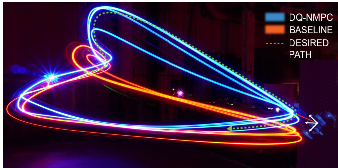
Fig. 1. Trajectory tracking experiment comparing Dual-Quaternion NMPC and Baseline NMPC. Green lines indicate the desired trajectory, blue lines show the system's evolution under the DQ-NMPC controller, and orange lines represent the results obtained with the baseline NMPC.
