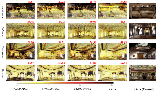
Fig. 5. Reconstruction error rendering of scene Auditorium , Ballroom , Courtroom , and Museum on the advanced set of the Tanks and Temples benchmark. The darker color indicates a larger reconstruction error and \tau denotes the per-scene point distance threshold. The top-right number denotes the F-score in % ( higher the better ).
