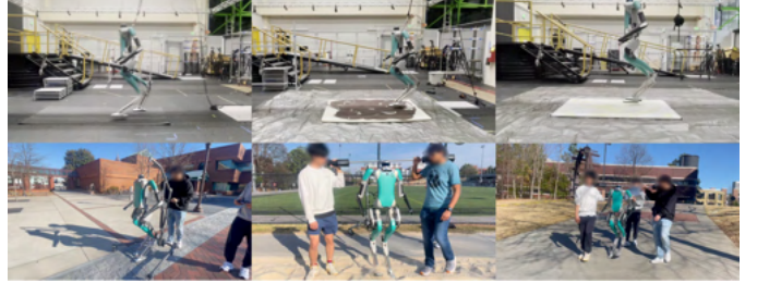
Fig. 1. Our Pre-training and Preservative Fine-tuning (PPF) framework achieves a forward velocity of 1.5 m/s while successfully traversing a whiteboard covered with poppy seeds or olive oil, as well as diverse outdoor terrains, including hills, uneven surfaces, and sand.
