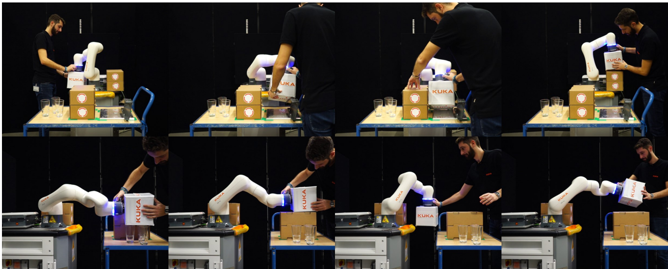
Fig. 9: Exploration phase through hand guidance of a KUKA LBR iiwa equipped with a cube-shaped exploration tool: front view (top row) and side view (bottom row). The corresponding swept volume is shown in Fig. 1.
