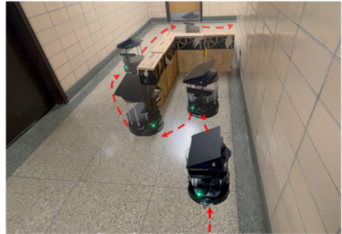
Fig. 9. An example of X-Nav overcoming local minima in a real-world experiment.
