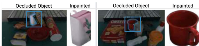
Fig. 3. In the image inpainting module, occluded objects (blue borders) are transformed into single fully observable objects.
