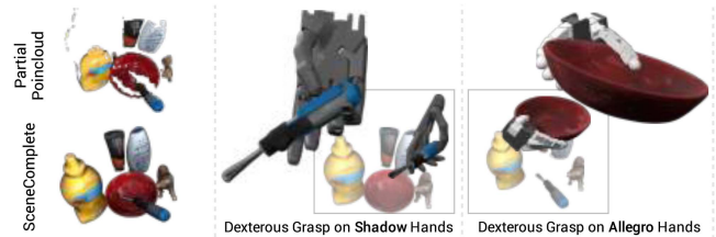
Fig. 7. We demonstrate dexterous grasps using both Shadow Hands and Allegro Hands [5] on objects from the GraspNet-1B dataset, highlighting improved manipulation of complex objects with complete 3D reconstructions.
