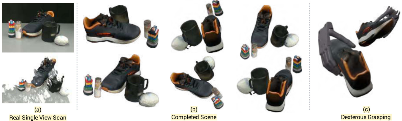
Fig. 1. (a) takes as input a single RGB-D image of a given scene, visualized here as a point cloud; (b) produces high-quality fully completed, accurately segmented object meshes in scenes with substantial occlusion and novel objects; and (c) enables downstream dexterous manipulation that requires accurate complete shape information.
