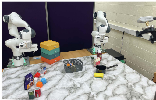
Fig. 3. Snapshot of the real-world experimental setup: two Franka Research 3 robotic manipulators positioned along with an external Intel RealSense D435i RGB-D camera.
