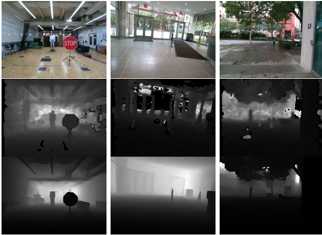
FIGURE 17. Qualitative results of depth completion. (Top) RGB inputs. (Middle) Raw stereo depth from the onboard sensor, which suffers from missing or noisy regions, especially around thin structures, glass, and foliage. (Bottom) Completed depth maps produced by our fusion module. The system recovers fine details, such as railings and branches, that are critical for collision avoidance but often missed by stereo matching alone. This enables safe navigation in visually complex environments.
