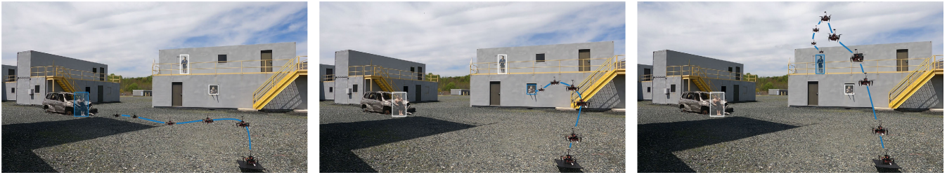
FIGURE 15. Impact of adaptive zoomed-in view multitarget scenes. In cluttered scenes with multiple visually similar targets (white), tracking can become unstable when relying on full-frame detection, often resulting in identity switches or drift. The adaptive zoom module addresses this by cropping tightly around the prompted target, suppressing distractors, and maintaining detection focus. Shown here are drone trajectories (blue) for three separate trials, each prompted to track a different mannequin. NOVA successfully adheres to the correct target in all cases.
