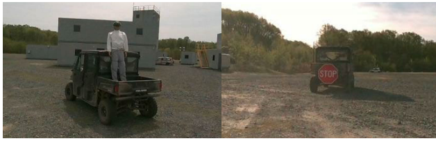
FIGURE 8. Targets used for tracking. Experiments use either a 1.8-m mannequin on an ATV or a 0.8-m reflective stop sign. The mannequin simulates a human presence, while the stop sign adds glare and reflection challenges. The ATV moves the targets dynamically at speeds up to 50 km/h.
