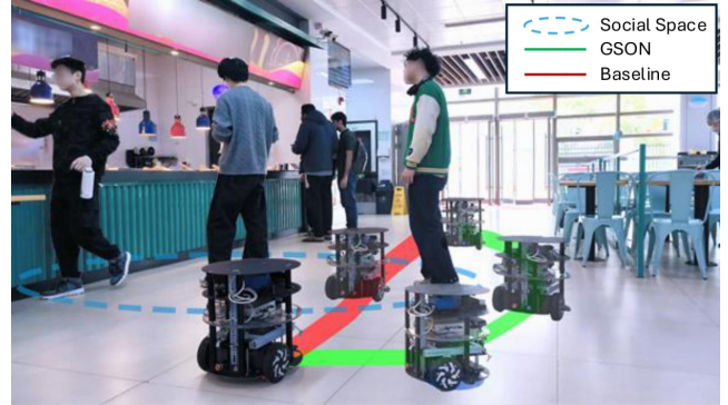
Fig. 1. Example of a social navigation scenario: Rather than walking between two individuals in a queue, the robot correctly identifies the social context and navigates around the queue to avoid disturbance.
