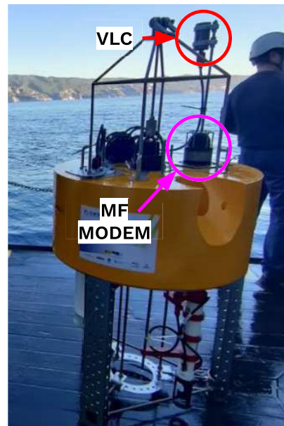
Fig. 7. Lander 1 equipped with a VLC and a MF modem.
