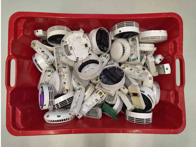
Fig. 1. A batch of heat cost allocators and smoke detectors. The variety of designs and different states of damage make the removal of batteries difficult.
