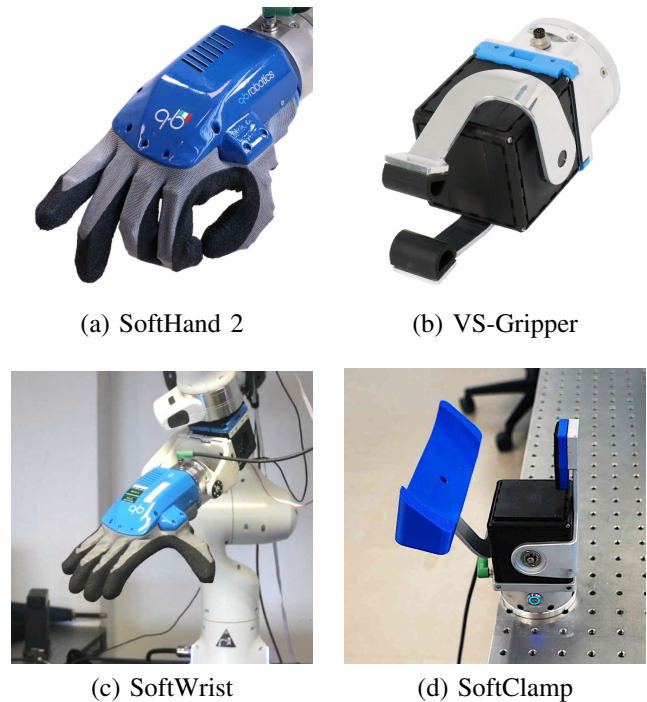
Fig. 6. Soft robotics tools developed and adapted to the problem of disassembly of electronic waste.
