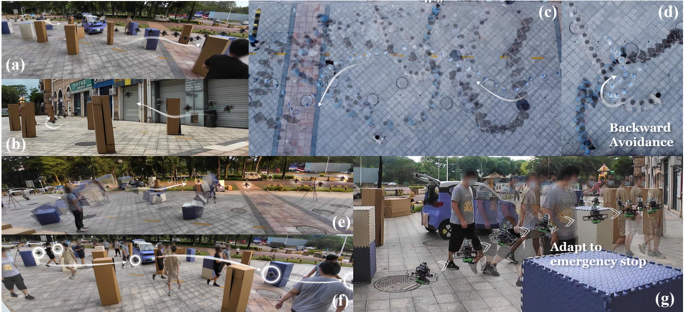
Fig. 8. Real-world experiments. (a) Traversal through a box environment. (b) Agile flight with high reference acceleration input. (c) Frequently interacting with pedestrians. (d) Highlight of a backward avoidance when performing a similar experiment to (c) in a lower agility. (e) Reacting to fast-moving objects. (f) Navigation among static and dynamic obstacles. (g) Details of adapting to an obstacle emergency stop in experiment (f).
