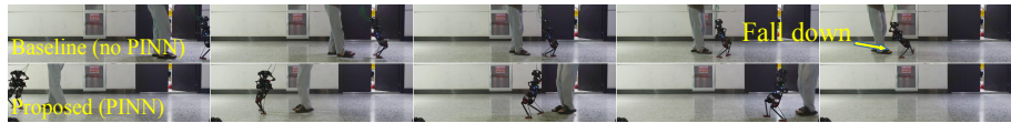
Fig. 9: Stability comparison of the robot at maximum reverse speed under two sim-to-real transfer methods.
