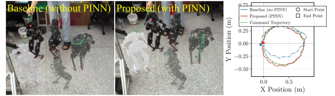
Fig. 7: Tracking performance of BRUCE following a circular reference trajectory under two different sim-to-real transfer methods.
