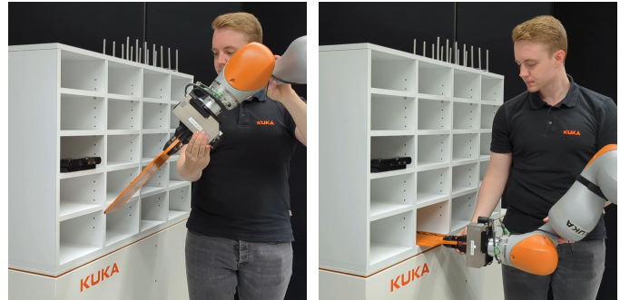
Fig. 1. Experimental setup for a scenario with task variance. Demonstrations are provided through hand-guiding. The variable motion skill includes picking a board out of the non-stationary rack, holding it in front of the camera (left) and inserting it into the shelf in different slots (right).
