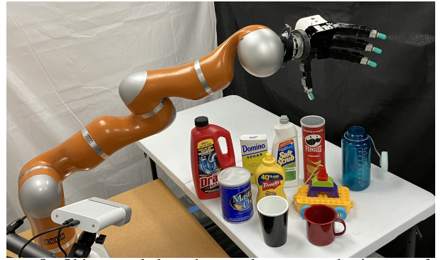
Figure 9: Objects and the robot used to assess the impact of our method on dexterous grasping.
