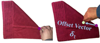
Fig. 3. Illustration of offset vectors. Left: grasping the Endpoint Belonging to the Connecting Part. Right: grasping a Point Belonging to the Upper Layer.
