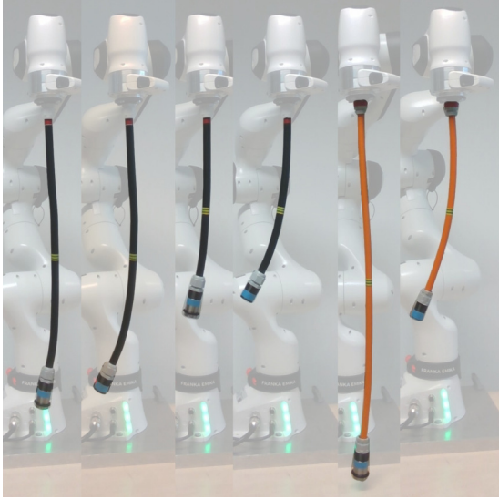
Fig. 3: The test objects used in the experiments, OB1-OB6 from left to right. These are high-voltage electric cables used in the context of the electric car industry. The cables end with a plug connector.
