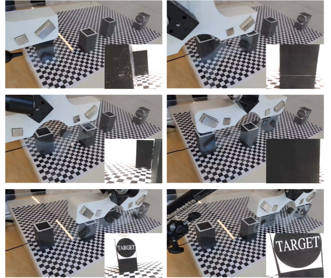
Fig. 14. Open-loop telemanipulation of the weight-compensated endoscope demonstrating obstacle avoidance from initial to target position.
