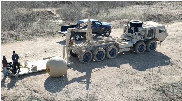
FIGURE 28. An aerial view of RoboBall III being deployed from Oshkosh HEMTT near crater.
