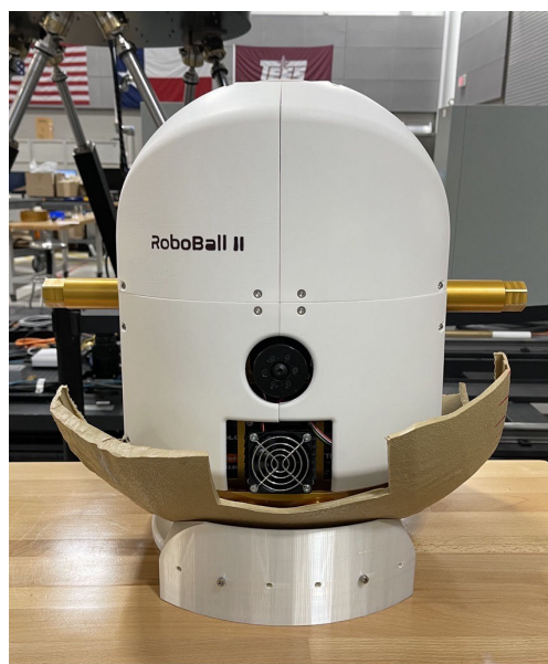
FIGURE 13. RoboBall II's inductive charger base and pendulum are mounted on its testing configuration.
