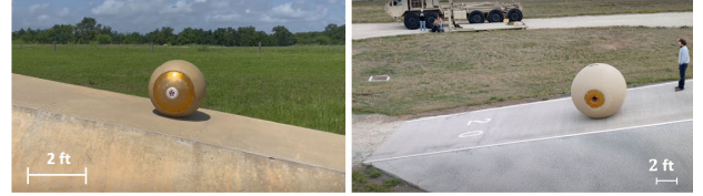
FIGURE 19. RoboBall II (left) and RoboBall III (right) actively descending a 15% grade incline and a 20% grade incline using variations of the same controller.
