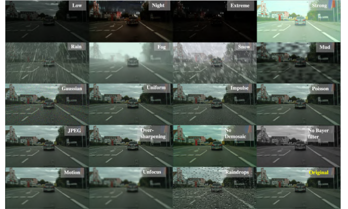
Fig. 1. Visual examples of the newly proposed degraded dataset (D-Cityscapes+) with 19 types of degradation, from top to bottom, are categorised as unfavourable light, adverse weather, internal sensor noises, motion blur, and distortion artefacts.
