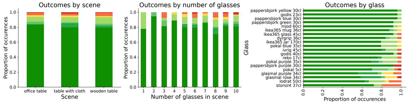
Fig. 5. Detailed performance analysis across 500 pouring trials. (Left) Outcomes grouped by scene; (Middle) Outcomes versus the number of glasses in the scene; (Right) Outcomes per glass type, sorted by success rate.
