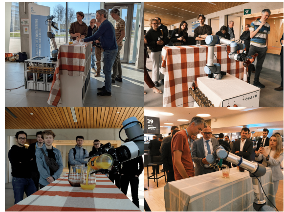
Fig. 6. The robot deployed in public events, autonomously detecting glasses and serving juice. Across multiple events, it successfully served over 200 drinks with 98.3% success in a 62-pour session.
