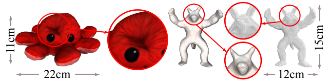
Fig. 9: Examples of reconstructed ground truth meshes for medium (Left) and small (Right) size objects in deformed states. Reconstruction of fine-grained details is a limitation of our current setup (close-up views on the Right).
