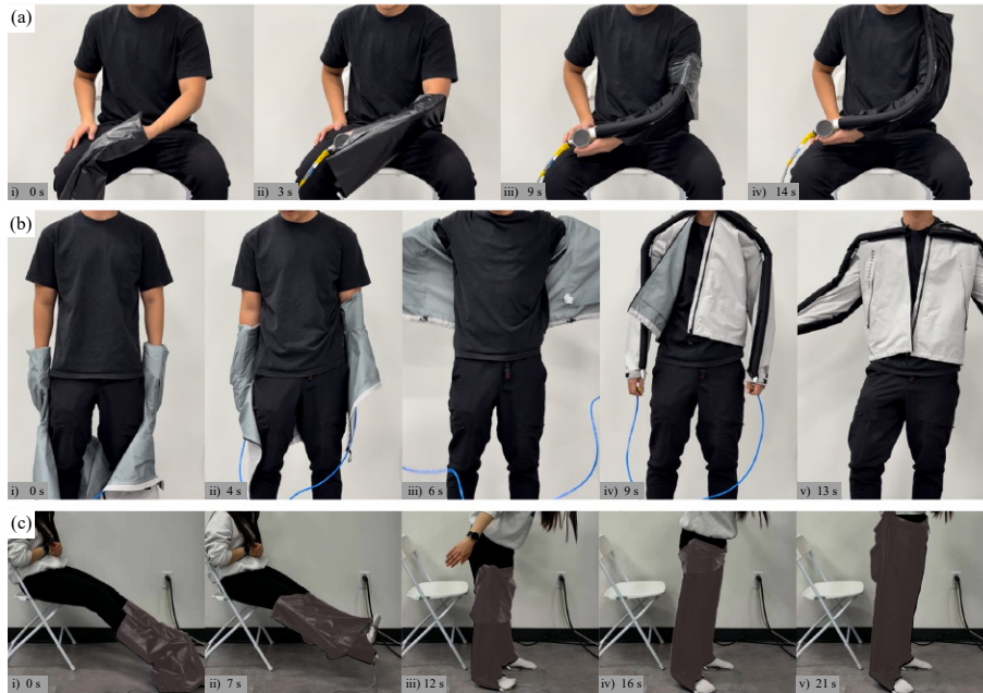
Fig. 8. Self-wearing demonstration using the SWAG system. (a) Basic donning operation using a sleeve-type prototype actuated by an automated base station. (b) Jacket donning demonstration with the SWAG integrated as an active component of the garment. (c) Pants donning demonstration with the SWAG integrated as an active component of the garment (see the Supplementary Video).
