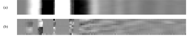
FIGURE 3. (a) Comparison of a raw B-scan containing k = 10 traces and (b) filtered result after applying background removal, dewow filtering, SEC gain, and wavelet denoising. Note that the direct wave bands are removed, and the deeper features (more rightwards) are more pronounced.
