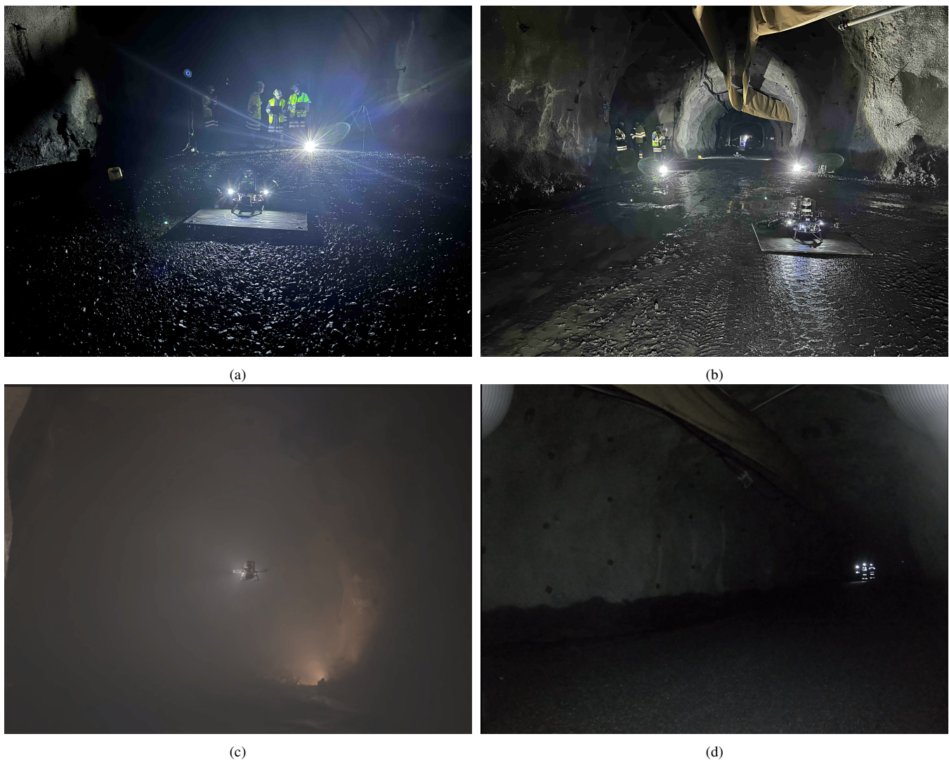
Fig. 1: The evaluation environment at a depth of over 500m in an active production area of the mine located in Kiruna, Sweden. (a) and (b) show the tunnel environment, with the aerial vehicles on the ground before a mission is initiated, (c) illustrates one of the many challenges for autonomy in a mining environment, flying in smoke-filled or dusty environments. Finally, in (d), a snapshot of an empty tunnel is presented to show the scale of the operating environment.
