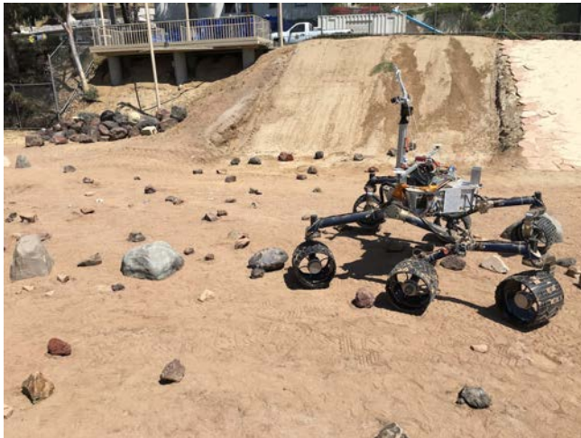
FIGURE 22. Scarecrow rover. It has a copy of the flight mobility hardware, and its weight on Earth is the same as Perseverance’s weight on Mars.
