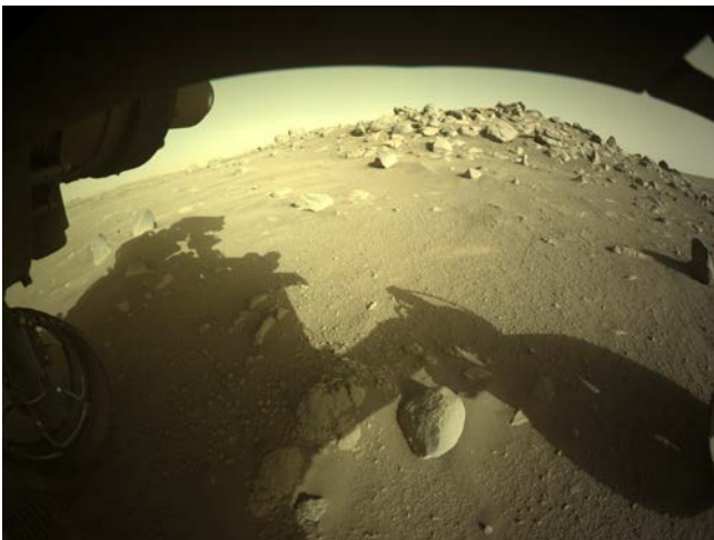
FIGURE 28. First guarded drive on Mars occurred on sol 107 (June 8, 2021), and successfully stopped before driving into the rock pile in front of the rover. This postdrive front HazCam view shows the rock pile is still well ahead of the rover’s stopping point.
