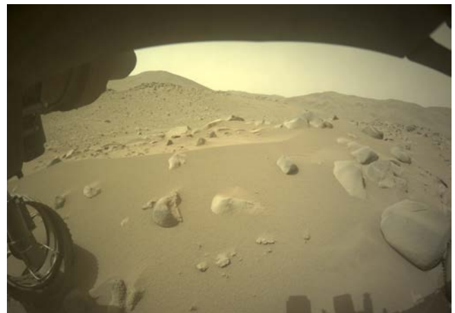
FIGURE 31. Front Hazcam from sol 1100, illustrating the rocky, sandy, higher tilt complex terrain region that ENav was unable to navigate using its initial conservative parameter settings from sols 1096 to 1159.
