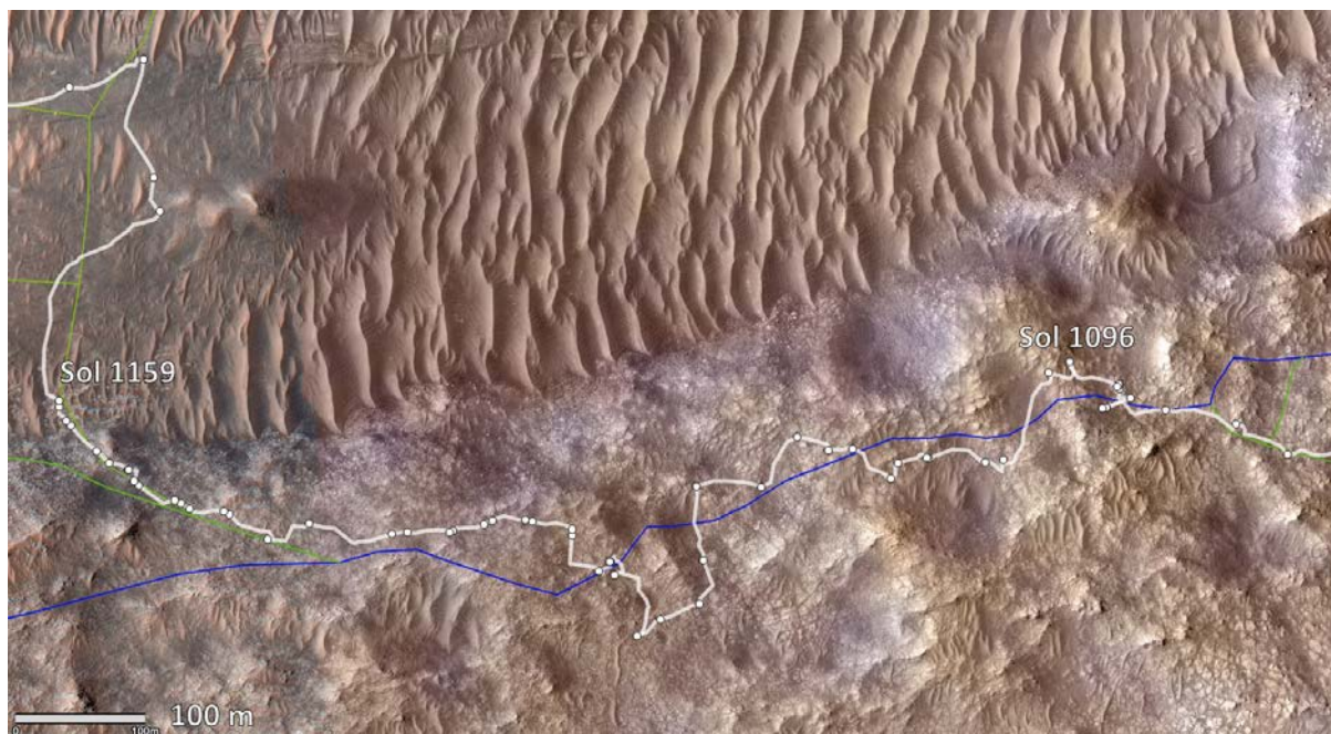
FIGURE 32. Orbital view of the complex terrain region through which AutoNav could not find a safe route. Instead, all drives from sol 1096 to sol 1159 were human-directed and, therefore, limited in distance by local terrain occlusions. Image credit: NASA/JPL-Caltech/University of Arizona/USGS.
