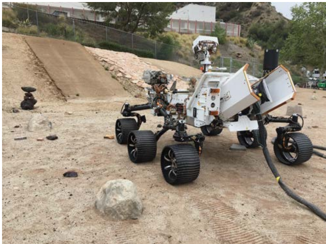
FIGURE 23. VSTB rover, which has mostly identical hardware (including avionics and mobility) and software to the Perseverance rover.
