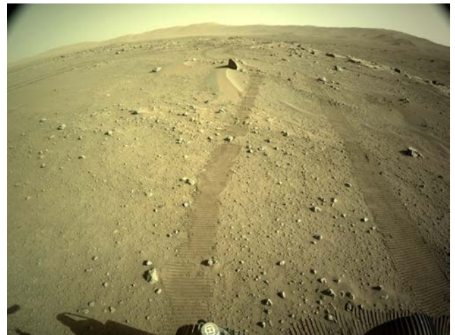
FIGURE 29. Second AutoNav checkout drive on Mars occurred on sol 122 (June 24, 2021), and was the first one to encounter (and successfully avoid) an obstacle. This postdrive NavCam view shows the rover tracks skirting around the obstacle.
