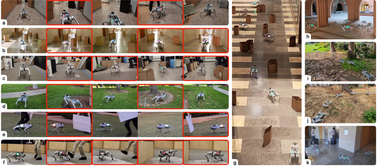
Fig. 1. Our proposed observation-conditioned reachability-based (OCR) safety-filter framework automatically safeguards different controllers in diverse settings for agile planar navigation tasks without a priori access to the controllers or environments . A trained OCR value network governs the switch between nominal and filtered control using an onboard LiDAR sensor. The framework successfully safeguards a variety of high-level planners, including (a) learning-based, (c, f, k) model-based, (b, d, g, h, i, j) human teleoperated, and (e) naive planners, on top of different low-level locomotion policies, including (a, f, i, j, k) learning-based and (b, c, d, e, g, h) model-based policies. Safety is maintained despite (a, b, c) narrow corridors, (d, i, j) rough terrains, (e, k) dynamic obstacles, (f) external disturbances, and (h) collision-seeking human teleoperation.
