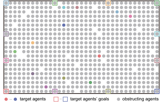
Fig. 9. Simulation environment for Experiment 3. The grid size is 35 \times 21 . Obstructing agents occupy 95% of the cells.
